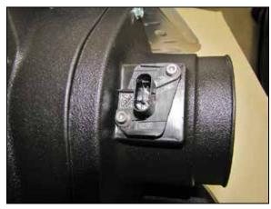
10. Remove the intel air temperature sensor from the factory housing and install it into the AEM® housing using the provided hardware.
