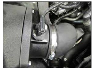
12. Reconnect the inlet air temperature sensor electrical connection.
