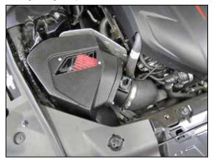
11. Install the provided coupler onto the turbo inlet. Install the AEM® filter housing assembly into the vehicle so the mounting studs engage the factory mounting grommets. Connect the intake coupler to the housing and tighten the hose clamps. NOTE: on vehicles equipped with a strut tower brace, reinstall the brace and secure with the factory hardware.
