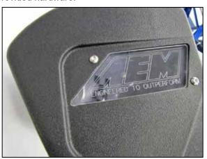
5. Install the AEM® window into the AEM® air filter housing and secure with the provided hardware.
