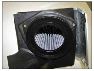
8. Install AEM® air filter into the filter housing as shown.
