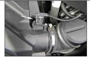
2. Disconnect the inlet air temperature sensor electrical connection and loosen the hose clamp that secures the factory intake tube to the air filter housing. Pull up the air filter housing to release it from the mounting grommets and remove it from the vehicle. NOTE: On models that are equipped with a strut tower brace use a E14 reverse TORX socket or a 7/16" 12 point socket to remove the bolts that secure the strut brace.
