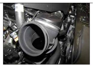
3. Loosen the hose clamp that secures the intake tube to the turbo inlet and then remove the intake hose from the vehicle.
