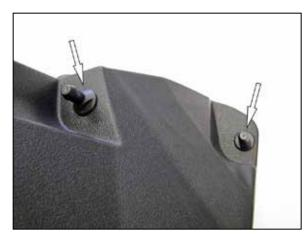
4. Install the two provided mounting studs onto the bottom of the AEM® air filter housing using the provided hardware.
